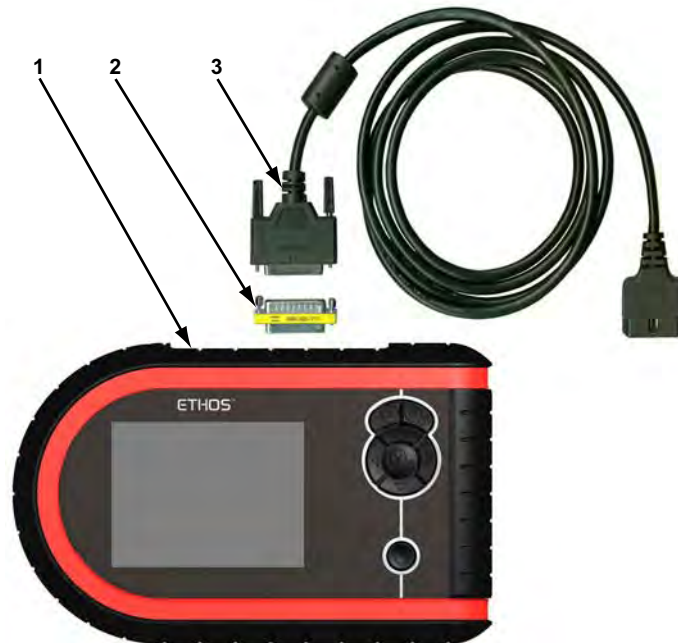
Figure 3-2 Data cable connections
